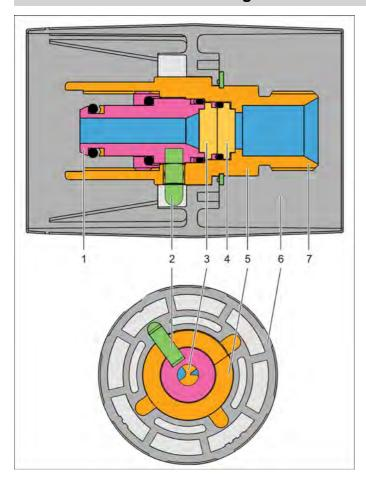
Water flow with opening angle 0° - 90°
